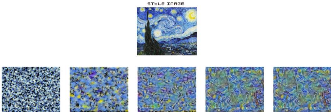
Figure: Reconstruct the style from a style representation built on different subsets of CNN layers: \{\text{conv1}_1\} , \{\text{conv1}_1, \text{conv2}_1\} , \{\text{conv1}_1, \text{conv2}_1, \text{conv3}_1\} , \{\text{conv1}_1, \text{conv2}_1, \text{conv3}_1, \text{conv4}_1\} , \{\text{conv1}_1, \text{conv2}_1, \text{conv3}_1, \text{conv4}_1, \text{conv5}_1\} .
